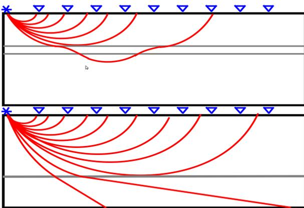
**Figure 4** Ray-tracing a long a layer velocity model. Ray-path trajectory depends on velocity variation. Model depth will affect ray trajectory and fold.
