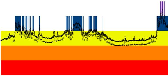
**Figure 3** Initial velocity model. First velocity 2000m/s, depth 200m, last velocity 6000m/s. Cell size 100m<sup>2</sup>.
