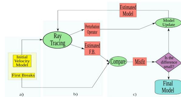
**Figure 1** Tomographic update loop: a) First-break picking and initial velocity model, b) Ray tracing, c) Model update
